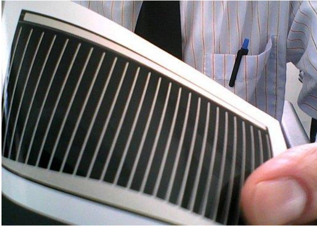
Figure: Thin CIGSe (Cu(In,Ga)(Se) 2 ) solar cell, produced at Solarion AG. Substate: Polyimid. source: https://en.wikipedia.org/wiki/Copper_indium_gallium_selenide_solar_cell
