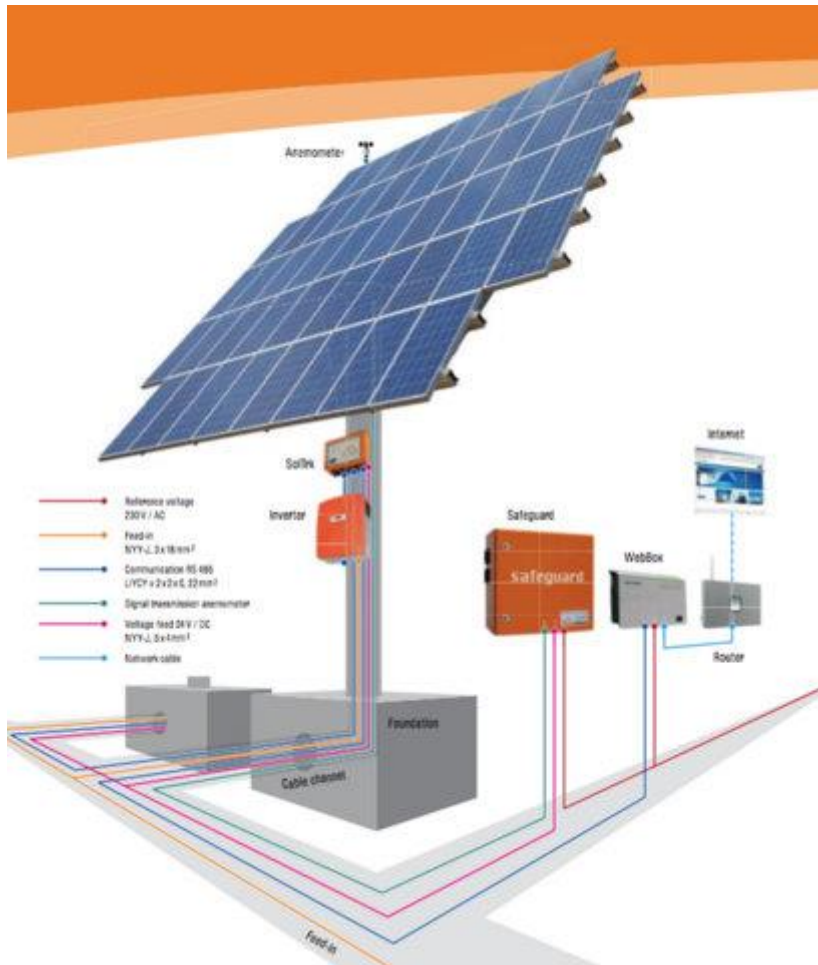
Figure: Dual Axis Solar PV Tracker. Connections and Cabling. source: https://eco-energ.co.uk/solar/solar-pv-tracker/
