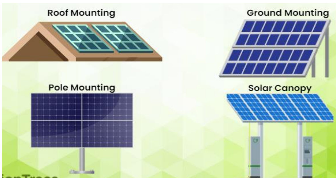
Figure: Ground-mounted photovoltaic systems offer a number of advantages over roof-mounted ones, source: https://8billiontrees.com/solar-panels/solar-panel-racking/
