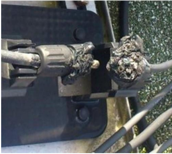
Figure: A cross-mating connectors from two different manufacturers potential points of arcing fault occurrence.
