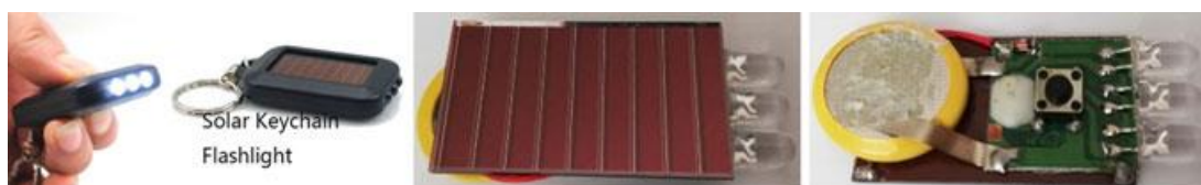
LED keychain torch with solar photovoltaic charge
