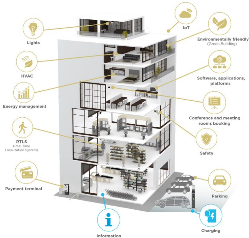
Figure 20 Representation of the needs a BMS controls.
