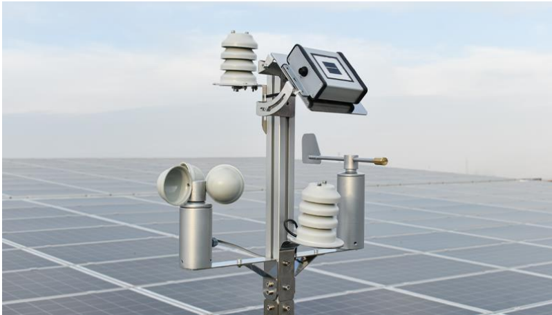
Figure: A meteorological PV Station source https://www.sevensensor.com/
