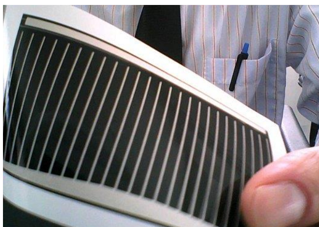
Figure: Thin CIGSe ( \text{Cu}(\text{In,Ga})(\text{Se})_2 ) solar cell, produced at Solarion AG. Substrate: Polyimid. source: https://en.wikipedia.org/wiki/Copper_indium_gallium_selenide_solar_cell
