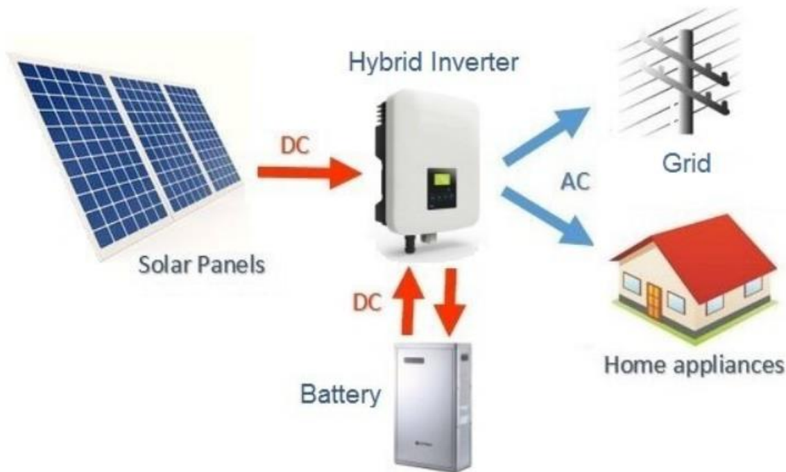
Figure: Depending on the mission of each inverter, a distinction is made between inverters that are connected to grid systems (grid inverters) or in stand-alone systems (stand-alone inverters). source: https://www.cleanenergyreviews.info/blog/what-is-a-hybrid-inverter
