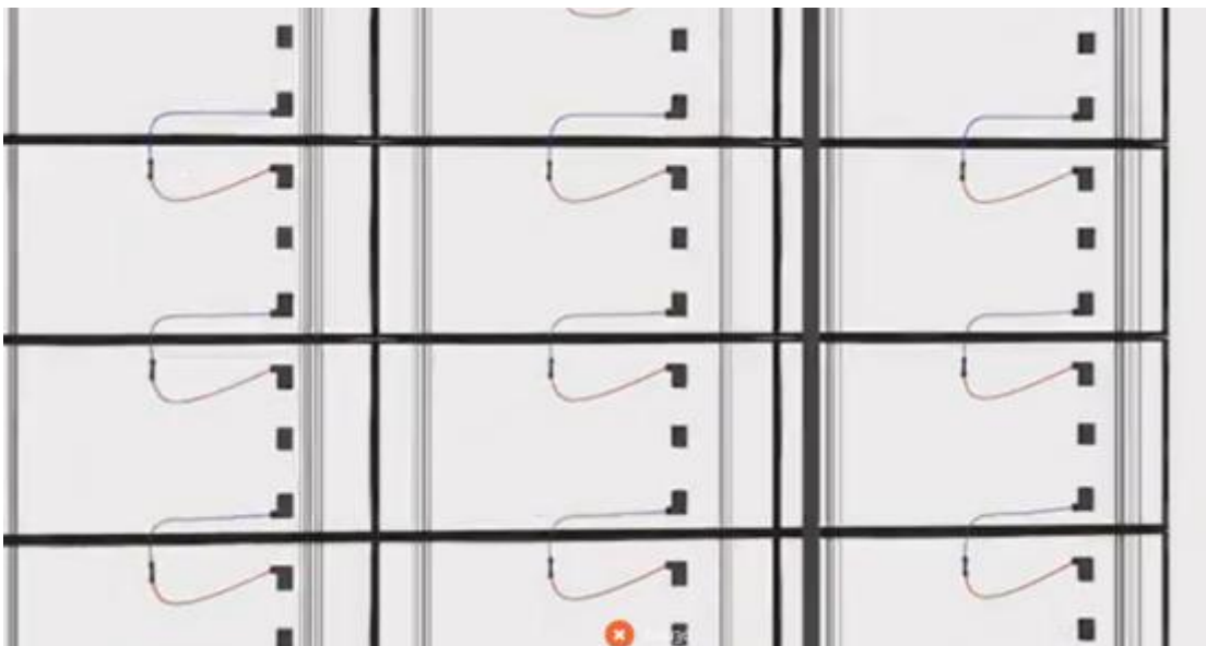
Figure: Connectors connected together in strings, source: https://www.mitrex.com/technology/
