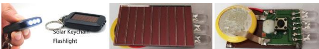
LED keychain torch with solar photovoltaic charge
