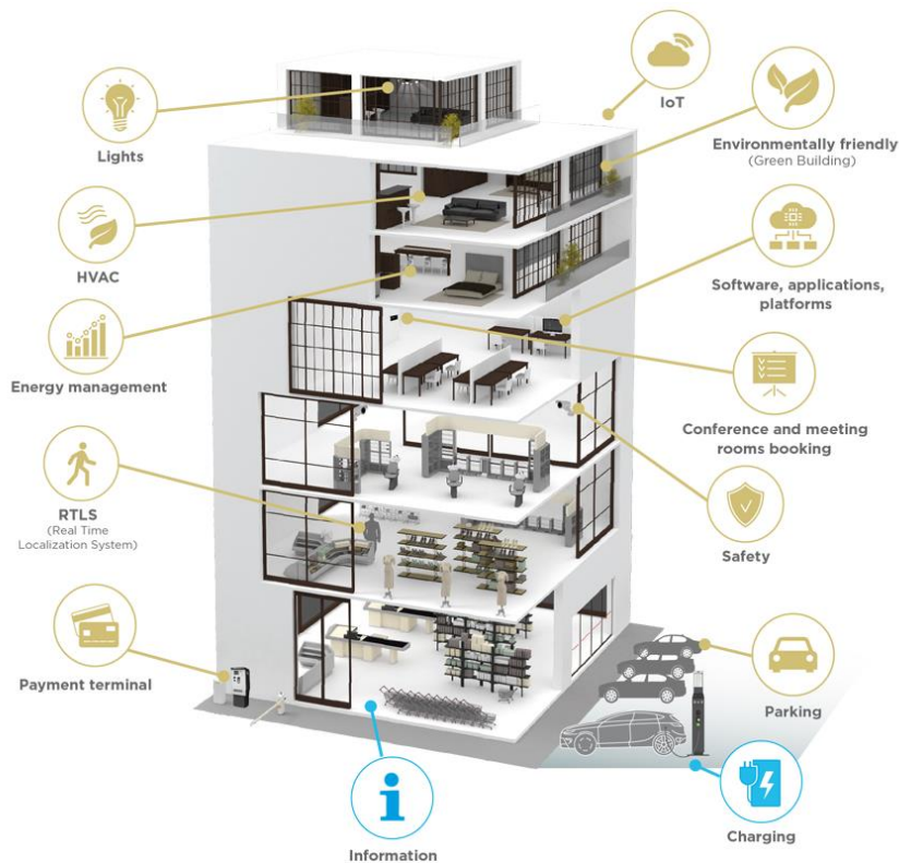
Figure 20 Representation of the needs a BMS controls.
